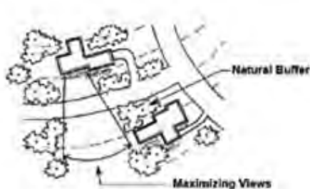
Exhibit 3.5 – Existing trees preserve the visual quality of the site and allow for natural screening.
